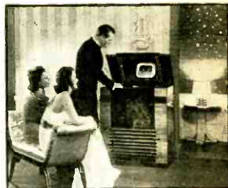
RCA Victor Television Receiver Model TRK 12. Has 12-inch Kinescope which reproduces an image 7½ x 9¾ inches on a mirror on the underside of the raised lid for indirect viewing. Reproduces images in unusually fine detail. Utilizes 36 tubes in addition to Kinescope. Electric tuning for sound reception is provided for 9 stations. Cabinet is of fine matched woods, and measures 40½ x 34½ x 19½ ins. deep.
