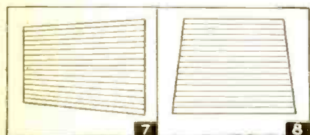
Figs. 7 and 8. Showing the effect of trapezium distortion caused by unbalanced sweep voltages. The line formation is exaggerated.
